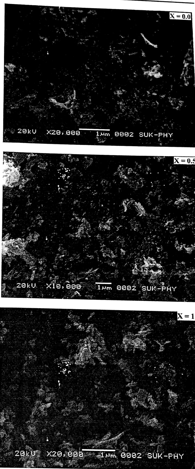
Fig. 5 SEM images of \text{Ni}_{0.65}\text{Zn}_{0.35}\text{Al}_x\text{Fe}_{2-x}\text{O}_4 , x=0.0, 0.5, and 1.0 samples
